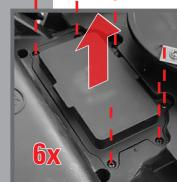
Loosen screws, remove cover
