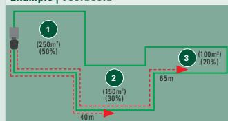
**i** Example for 10 cycles: In 5 random mowing cycles the robot mows area 1, in 3 it runs from the back of the charging station 40 metres along the limitation cable and mows area 2, in 2 it runs 65 metres along the limitation cable and mows area 3!
