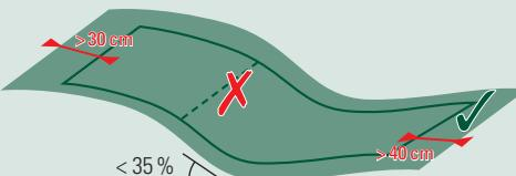
When laying the limitation cable on slopes, observe the required distances and maximum incline permitted! The corner of the limitation cable should be on a level surface.
